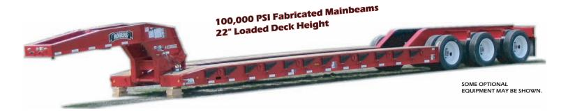
The ROGERS<sup>®</sup> **CENTURY™ CY50** – hassle-free hauling in a 50-ton capacity detachable goosneck trailer. It features fabricated main beams, the "No-Foot"<sup>®</sup> self-lifting gooseneck and a tapered front end to assist loading. It is designed for a 2/3 load concentration to easily carry the 50 tons in 16'-0" of deck, so you can focus on getting your equipment to where it is needed.
