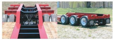
Lowered crossmembers in the rear frame make a "boom trough" - more space for excavator booms. Oak decking to the tires yields an extra foot of deck length. Light-weight outriggers on rear frame are used to tie-down loads. Each axle has spring-loaded parking brakes and a premium 4S/2M anti-lock braking system.
