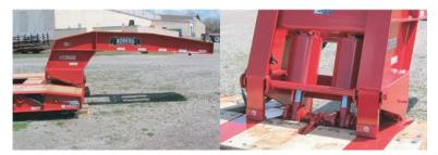
■ Exclusive "Croucher"® front with tapered beams hugs the ground for optimal loading stability and approach angle. Concealed beam hooks won't damage low ground clearance equipment. The powerful, low operating pressure "No Foot"® self-lifting gooseneck saves time and effort by lifting the rated load on any terrain and permits quick deck height adjustment to clear obstructions. Equipment can ride over the Scraperneck gooseneck to maximize use of the deck length.
