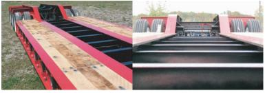
■ Unitized frame with main beams fabricated of 100,000 PSI steel. Heavy-duty, full-width cross members on 24" centers for longer deck life. Full 1 3/4" air-dried oak decking installed with carriage bolts and cupped washers for easy replacement. Removable swinging side brackets widen the deck to 10'- 6". Tested and certified lashing D's exceed today's load securement regulations.
